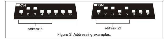
Five switches make it possible to assign addresses to 32 expanders (numbers from 0 to 31). Addresses of the expanders connected to one bus may not repeat, while the addressing sequence is optional. It is recommended to assign consecutive addresses, starting from zero, to expanders and other modules connected to one bus. This will permit problems to be avoided during extension of the alarm system.
